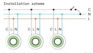
Control line C is used to control the switching on and off of the central LED in the presence of mains power (maintained or non-maintained mode).
