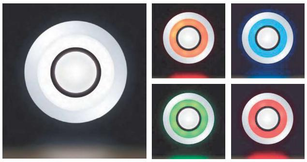
Matiz in maintained mode: in addition to the ambient LED crown in the desired colour, the central white LED is permanently lit. In emergency mode, the ambient LED crown is switched off and the central LED lights up brightly.
